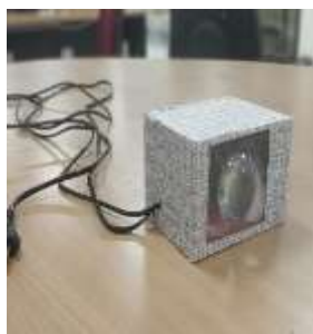
Transmitter module (10 x 6 x 7 cm)
